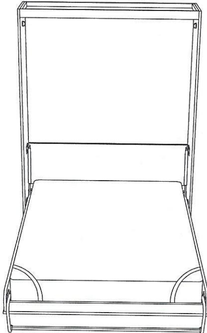
**NOTE:** When lowering the bed with the mattress it may seem very difficult. If the bed has too much power, i.e. - wants to close - you can easily decrease your bed's lifting power by using a socket wrench or driver. Turn the Hex Head to the right to move the ball stud to a smaller number - from five to four, or four to three. Be sure to adjust BOTH SIDES equally.
